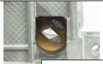
Locking Washer Installation Locations.
